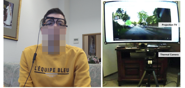
(a) Participant wearing the Pupil Labs eye tracker while watching projection screen placement. (b) Thermal Camera and video stimuli.
